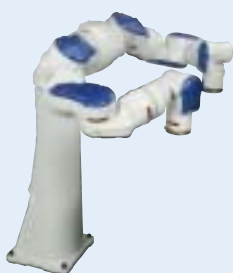
MOTOMAN-SDA5D/F Payload: 5 kg/arm (10 kg/dual arms)
