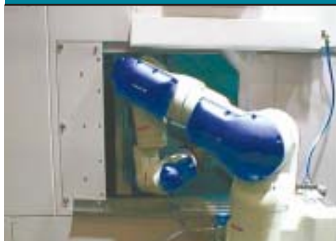
Attachment and Removal of Workpieces for NC Machines
