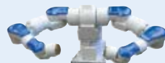
MOTOMAN-SDA20D/F Payload: 20 kg/arm (40 kg/dual arms)
