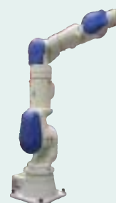
MOTOMAN-SIA30D Payload: 30 kg
