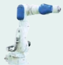
MOTOMAN-SIA50D Payload: 50 kg
