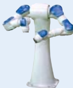
MOTOMAN-SDA10D/F Payload: 10 kg/arm (20 kg/dual arms)
